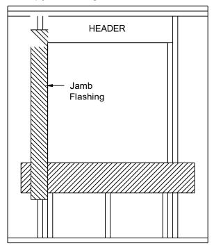
3. Install window flanges over sill and jamb flashings. Seal window per manufacturer's recommendations.
