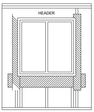
4. Install head flashing over windowflange. Extend 1" beyond outer edge of jamb flashings.
